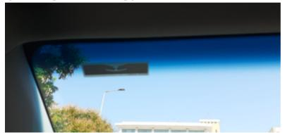
⚠ It's highly recommended that the location will be tested before sticking the UHF label to the windshield
